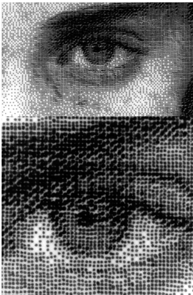
Figure 10. Photomicrograph of image printed using spot volume modulation.
